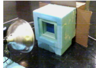
Figure 1: Trombe wall design. Sunlight passes through glazing and warms an air layer. Heat is transferred through a thermal mass made of high heat capacity material and into the living space.
